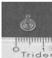
Fig. 2 Photography of the glass sample holder proposed in the present work. Reference scale in cm starting temperature (5–20°C) and the sample holder geometry. All the measurements were performed under dynamic nitrogen atmosphere with a gas flow of 50 mL min -1 .
